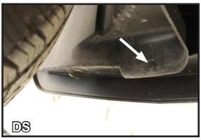
2. Remove the push pin that is located on the lower portion of the backside of the fascia, directly in front of the tire, using a flat screwdriver.
