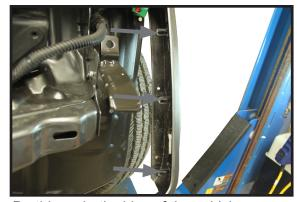
3. Holding the wheel well liner back, remove the three (3) clips. Do this on both sides of the vehicle.
