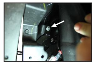
4. With the wheel well liner still pulled back, use a 10MM socket to remove the bolt. Do this on both sides of the vehicle.
