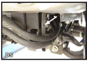
7. On the driver side only, move the coolant lines down and remove the push pin.
