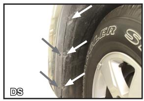
1. Remove the three (3) push pins located in the wheel well area of the vehicle using a flat screwdriver. Then remove the two (2) pop rivets.
