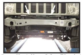
6. Press down gently on the plastic guard located beneath the grill in order to prevent damage to the guard.
